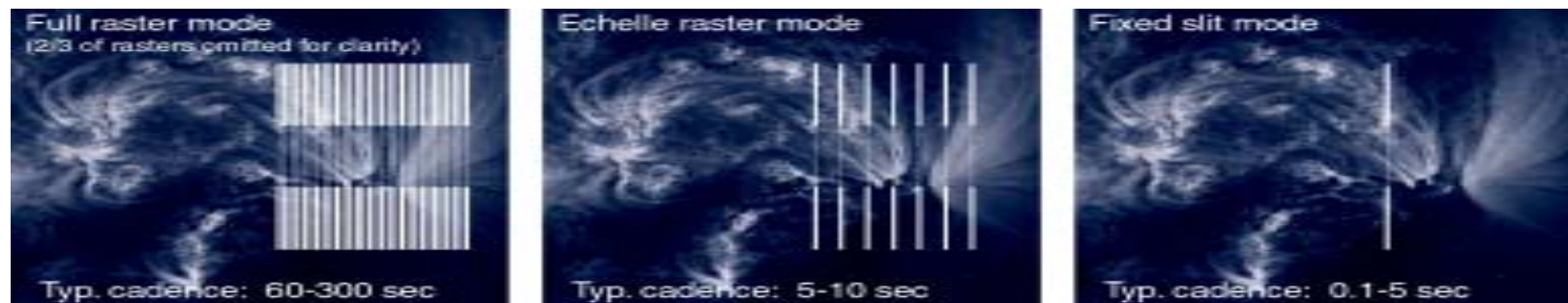
Figure 3: EUV Spectrometer Observing modes. Slit positions for the three principal observing modes are depicted, to scale, on a TRACE 171Å 200x200 arcsec 2 image showing coronal “moss” under an active region. Cadences are given for typical line selections and exposure times for each mode. Slit exposure times are typically 1-2 seconds for bright lines (used in the echelle scan); 1-5 seconds for a broader line selection (in the full scan).
