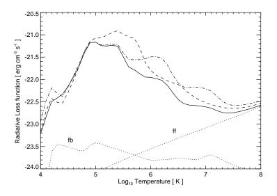
Figure 2. Radiative loss curves derived with CHIANTI assuming different abundances. The solid line is for solar photospheric abundances (Anders & Grevesse 1989), the dashed line noble gas enhanced abundances (Drake et al. 2001), and the dash-dot line solar coronal abundances (Feldman et al. 1992). The dotted lines indicate the contributions of free-free (ff) and free-bound (fb) continua.
